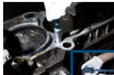
Length about 19cm with 3-15mm measuring range of bore diameter
