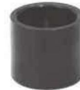
Locating repeatability will determine if one primary and one secondary or two primary liners are needed. With two primary liners, repeatability of ±0.013mm can be maintained if the two holes for receiver bushings are held to a centerline distance of ±0.005mm tolerance.
