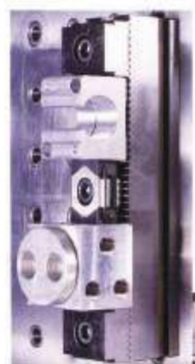
OK-VISE low-profile clamp is flexible to operate on different pallets.
