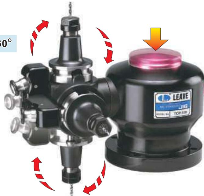
4pcs of M10x40mm bolt can be fastened from the top of the mounting flange or 4pcs of M12 bolt can be fastened from the bottom of the mounting
