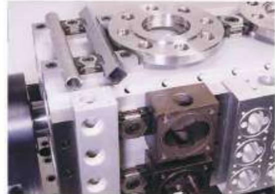
Accurate machining needs a free operative clamping unit. OK-VISE is a good solution for reaching such target because it is locked firmly in every direction as it is tightened down and this cuts out all possibilities of measurement error due to sliding.
